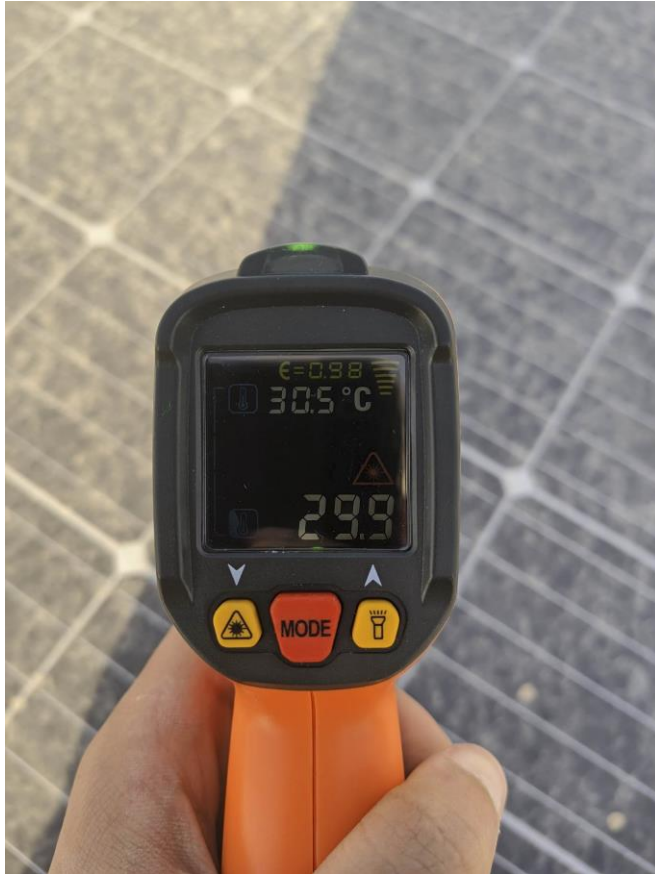
Figure 7.4 Temperature reading of the modules during operation
