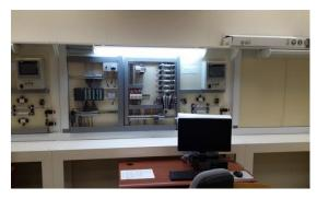
In this lab the student is introduced to different electric, optical, pneumatic and electronic sensors, and actuators. Furthermore, the student trained how to connect those units mechanically and electrically together using PLC or PC as controller. Moreover, the students are trained how to program PLC/PC to control these integrated electric-mechanical systems.
