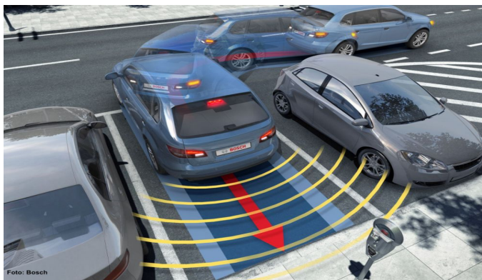
Figure 2.15 : Backup warning system
