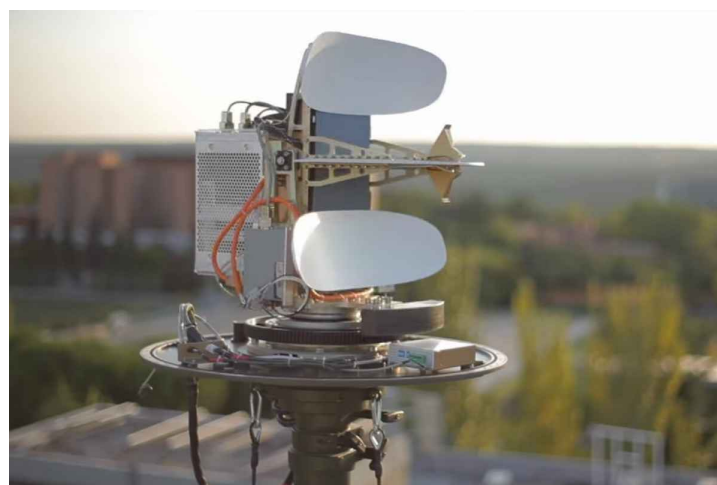
Figure 2.18 : The FMCW-Radar ART Midrange uses separate offset antennas for transmitting and receiving
