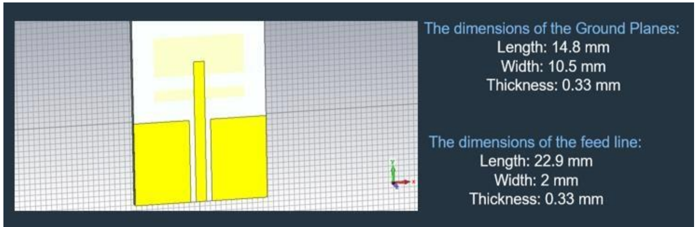
Figure 4.2: Ground planes and feedline (copper).
